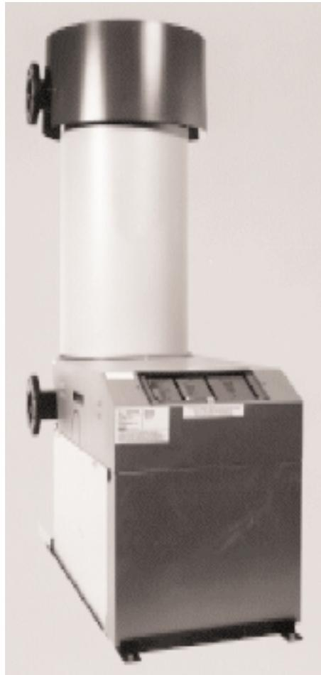
A modulating/condensing fuel-fired water heater or hydronic boiler can avoid losses associated, in conventional units, with cycling at less than full load and with unrecovered latent heat of water produced in the combustion process. A system which incorporates features that minimize cycling by modulating fuel and air flow to the combustor and that recover additional
